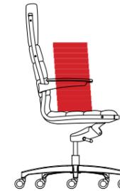
**VERTICAL STATIC LOAD ON THE CENTER OF THE ARMREST**
